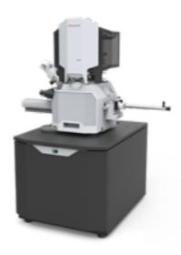
The Aquilos Cryo-FIB for preparing cryo-lamella Samples for high resolution 3D tomographic imaging
